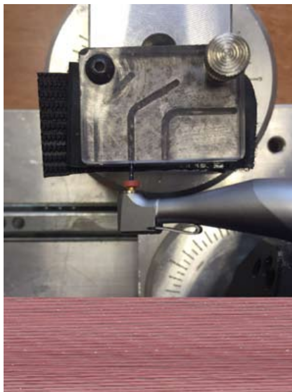
Figure 1. The testing device for cyclic fatigue.
