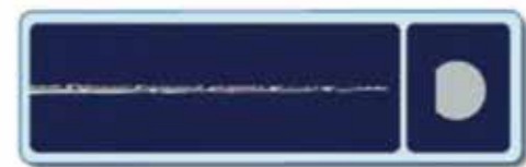
Figure 2: The "D"-shaped cross section of the Mani D Finder
